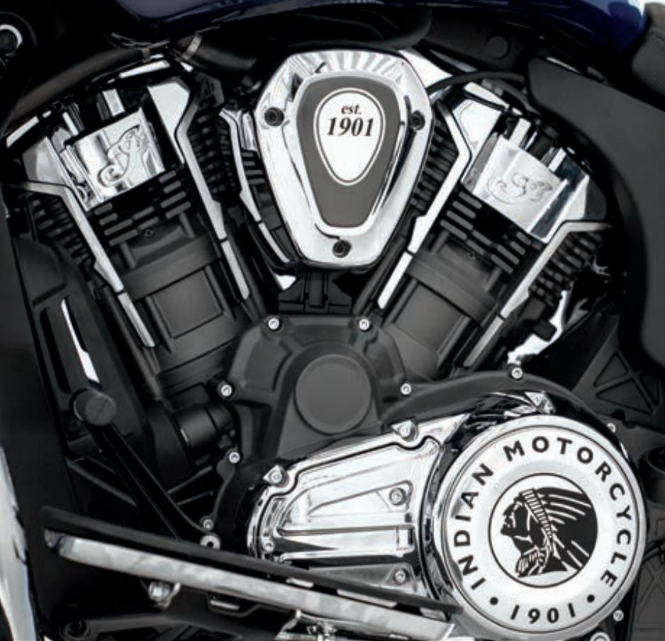
Our all-new liquid-cooled PowerPlus V-twin is the most powerful engine in its class. With overhead camshafts and four valves per cylinder delivering a blistering 122 hp and 128 ft-lbs of torque, it redefines American performance.
